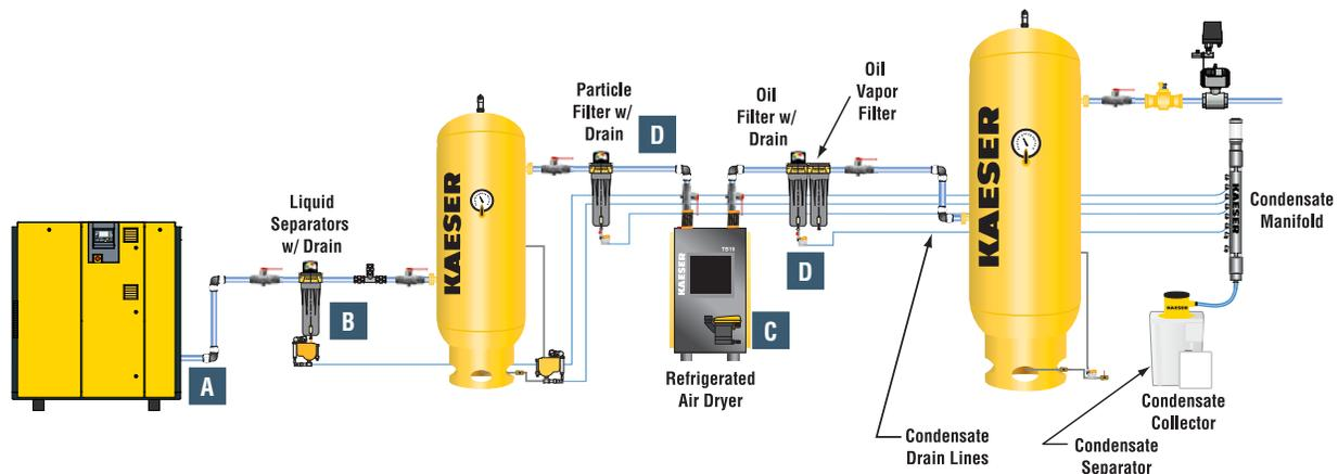
NOTE: Use AMD 6550 or Eco-Drain series with receiver tanks.
