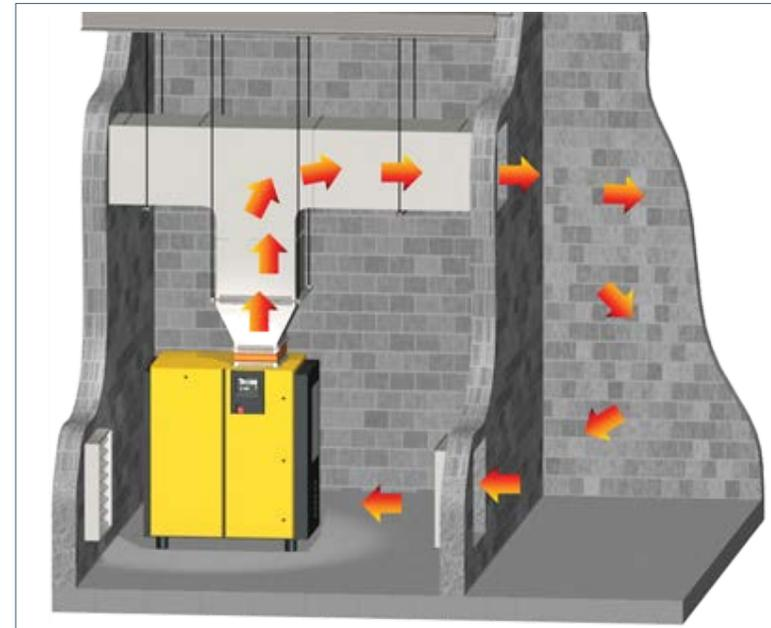
The diagrams on the following pages provide some basic hints for proper ventilation.
